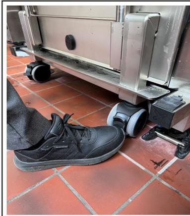
Ensure the wheels are securely **locked** whenever the trolley is inside the oven or not in motion.
